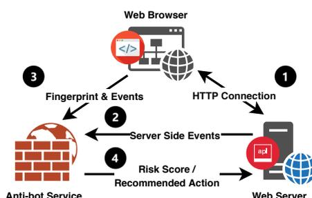
*Fig. 1: High-level architecture of Anti-bot services*
